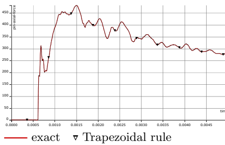
Fig. 17. Sample curves for trapezoidal rule, h = 2 \cdot 10^{-6} , nonsmooth friction law
