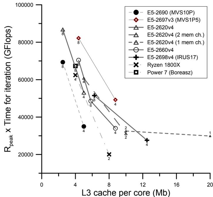
Fig. 3. The dependence of the  $R_{peak}\tau_{iter}$  parameter on the L3 cache per core.
